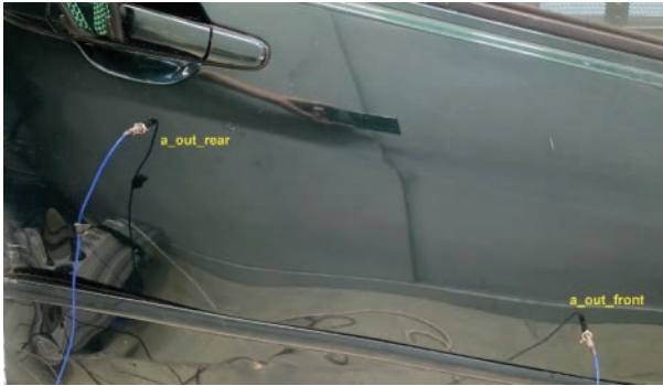
Figure 3: Location of sensors in outside panel
