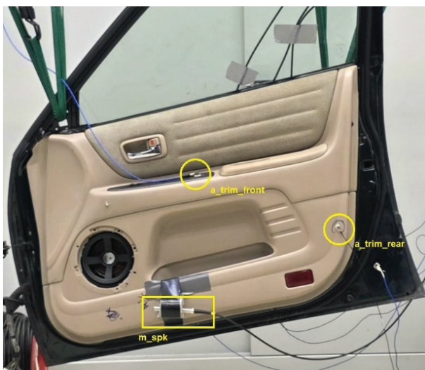
Figure 2: Location of sensors in door trim
