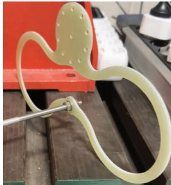
Figure 3: The finite element-designed spring.
